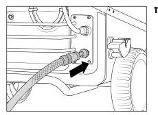
11. Connect water hose to water inlet (minimum requirements; 5 m hose length, cross-section ¾", 10 bar). The highpressure cleaner may be connected to a water mains (1-10 bar pre-pressure) with either cold or hot water (up to 60 °C). The therm-1-series provides the opportunity of sucking in water out of a container (see direct suction).
