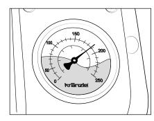
Having closed the trigger gun with safety catch, the high-pressure cleaner must shut down and the stainless steel pressure gauge must show the permitted deactivation pressure (see rating plate). If not shut down and the stainless steel pressure gauge continuously shows full pressure (device does not switch to bypass), this could be due to leakage at the high-pressure pump, at the pressure switch, at the high-pressure hose or at the trigger gun with safety catch.
