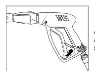
Apply the safety catch on the safety trigger gun after each use in order to prevent unintentional spraying!
