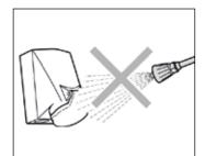
Never direct the high-pressure jet at power sockets or any other electrical installations! Within the working area, all live parts are to be protected from both water jet and spray mist.
