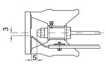
For a smooth ignition, the setting of the ignition electrode must be controlled regularly.
