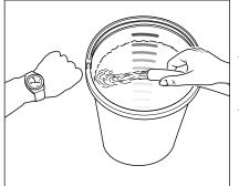
Lack of water occurs more often than you probably believe. The more powerful a highpressure cleaner is the greater is the danger that a lack of water occurs. If there is only an insufficient amount of water available, cavitation (water-gas mixture) arises inside the high-pressure pump, which is normally noticed too late or even not at all. **The highpressure pump will be destroyed.** Please check the available quantity of water by filling a bucket with liter scale for one minute.
