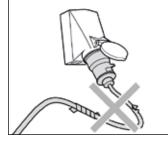
Only use a power supply cable in perfect working order! Do not damage or improperly repair the power cable (tearing, squeezing, running over, ...).
