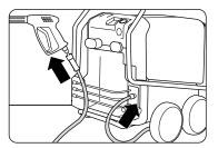
**Step 1:** Screw high-pressure hose down and pressuretight using safety trigger gun and lance.
