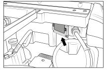
High-pressure cleaner turns There is an overpressure sensor on the rear of the control cabinet inside the highpressure cleaner.
