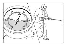
The stainless steel pressure gauge shows full pressure, but from the nozzle comes only little water or no water at all.
