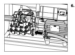
Connect water hose to water inlet (minimum requirements; 5 m hose length, cross-section <sup>3</sup>/<sub>4</sub>", 10 bar). The high pressure cleaner may be connected to a water mains (1-10 bar pre-pressure) with either cold or hot water (up to 60 °C). The WS-RP/WSC-RP-series provides the opportunity of sucking in water out of a container (see direct suction).
