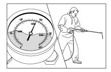
The stainless steel pressure gauge shows full pressure, but from the nozzle comes only little water or no water at all.
