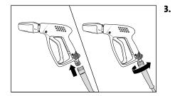
Mount the grey rotating screw connection of the high-pressure hose onto the trigger gun incorporating a safety catch. Afterwards screw together ensuring a snug and pressure-tight fit.
