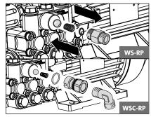
Remove check body and check O-Ring for soiling or damage. Also check seal seat inside pump housing for soiling or damage.
