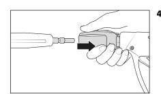
**4.** First pull back the retaining sleeve of the safety trigger gun, then insert lance into the plug coupling sconnection of the safety trigger gun.
