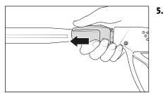
After insertion of the lance, release retaining sleeve and make sure that the lance is in a secure position.
