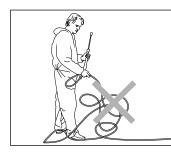
Never pull the high pressure hose if it has formed kinks or "nooses"! Never pull the high pressure hose over sharp edges!
