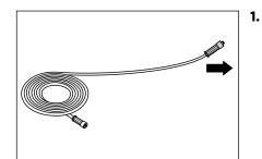
Unwind high pressure hose straight and without nooses. (When using high pressure hose extensions take care that the max. length of 20 m is not exceeded!) The high pressure hose may leave signs
