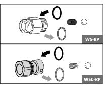
If sealing rings are defective replace O-rings at once.
