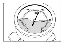
Having closed the trigger gun with safety catch, the high pressure cleaner must shut down and the stainless steel pressure gauge must show "O" bar. If not shut down and the stainless steel pressure gauge continuously shows full pressure, this could be due to leakage at the high pressure pump, at the pressure switch, at the high pressure hose or at the trigger gun with safety catch.
